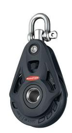
Core Blocks™ are a true all round solution. A tuned 2-stage bearing system provides excellent performance across the full working load range with an integrated thrust bearing feature and the resilience to handle high dynamic or static loads. Acetal sheave, alloy cheeks and stainless fixings complete the durable package. For reliability and a long service life, these blocks are the right choice for sheets, halyards and control line applications for cruising and racing.
