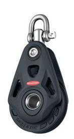
Core Blocks<sup>TM</sup> are a true all round solution. A tuned 2-stage bearing system provides excellent performance across the full working load range with an integrated thrust bearing feature and the resilience to handle high dynamic or static loads. Acetal sheave, alloy cheeks and stainless fixings complete the durable package. For reliability and a long service life, these blocks are the right choice for sheets, halyards and control line applications for cruising and racing.
