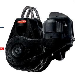
Total block load. Load on saddle not to exceed 15% of block load. ie. MWL 117kg (257lb), BL 234kg (514lb). Suitable for 6:1 system at rated block load.
